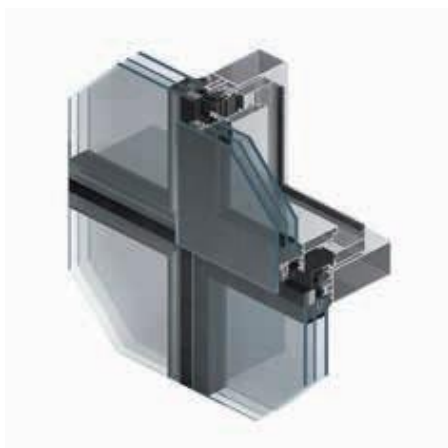
One of the most important advantages of this solution are the unusually economical shapes, which add lightness to the entire structure. Thanks to application of the most modern technology of structural gluing, based on gluing the outer glass panel to the aluminium frame with structural silicon, we have avoided the necessity to use any aluminium elements from the outside or any mechanical joints for fitting the glass panel.
